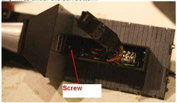
Place the lid on the toolbox, turn the Truck over, and attach the toolbox with the long screw that was removed.
