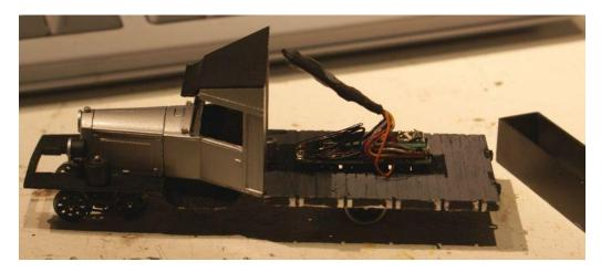
Replace the toolbox and screw it to the frame. This is the screw that is close to the cab. Be careful not to catch any wires under the box bottom.
