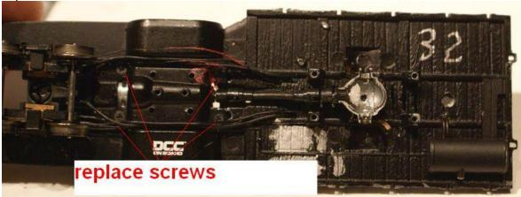
Assemble the rest of the drive line and connect to the motor drive line part. Drop the drive line in the rear transmission housing. Squeeze the two wheel pickups in slightly and insert the new wheel included in the package. Make sure you have contact between the wheel and the pick-up. If not, pull the wheel out and bend the contacts out slightly and repeat wheel install. Lube the gears if desired.
