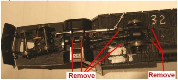
Remove the drive train (shown removed below). Then remove the four short screws and the longer back screw.
