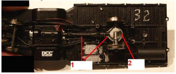
Replace the bottom of the transmission cover and the four screws.
