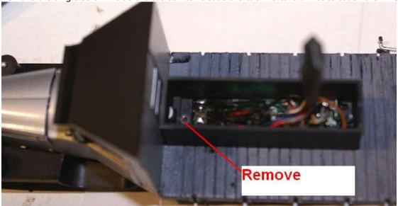
Turn the Truck back over and remove this last screw to release the lock on the back of the cab and remove the cab.
