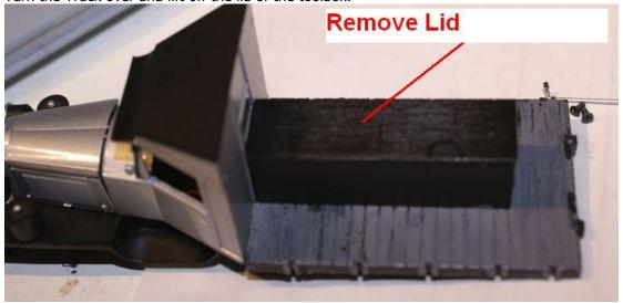
Remove the single screw inside the toolbox to release the cab. Be careful not to touch the wires for the decoder.
